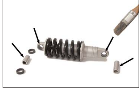
The bushings of the rear spring element need to be lubricated once a year.
