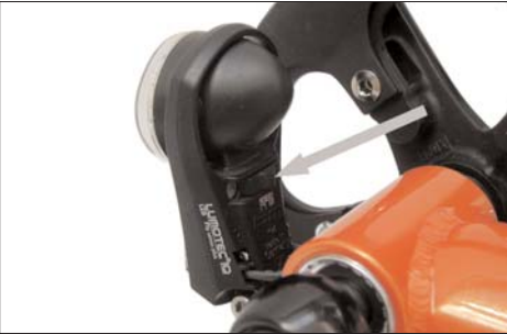
You switch on the hub generator lighting system with the integrated switch at the front light.
