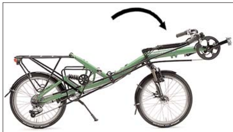
Bring right pedal to the front and fold handlebars forward
